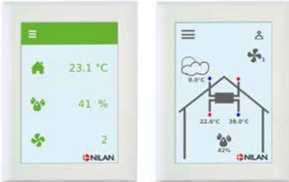
The VPR 120-560 range is controlled using its CTS 602i HMI touch panel, featuring a wide range of functions, e.g., menu-controlled operation, weekly programme settings, filter monitor with timer, fan speed adjustment, summer bypass, post-heating element control, error messages etc.
